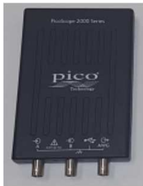
PicoScope 2205A 2 Channel, 25 MHz, 200 MS/s, 16 Ks Code PP966
